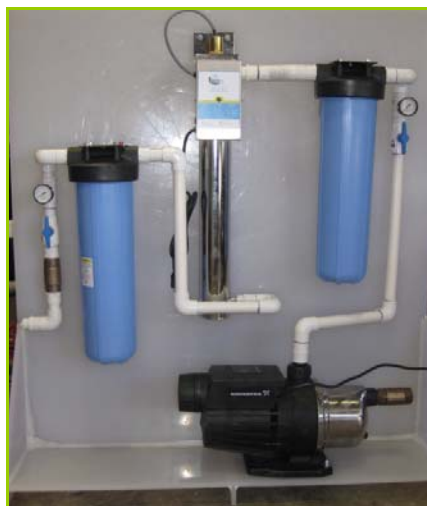
Purification Skid with Pump, 1-micron Filter, UV Light, and Carbon Filter
