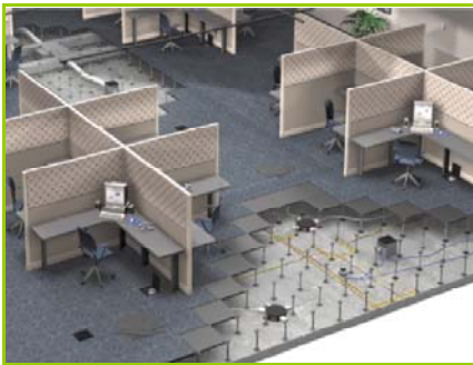
Raised Floor System during Construction
